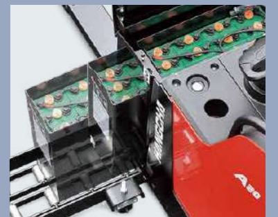
Side battery change is standard feature
